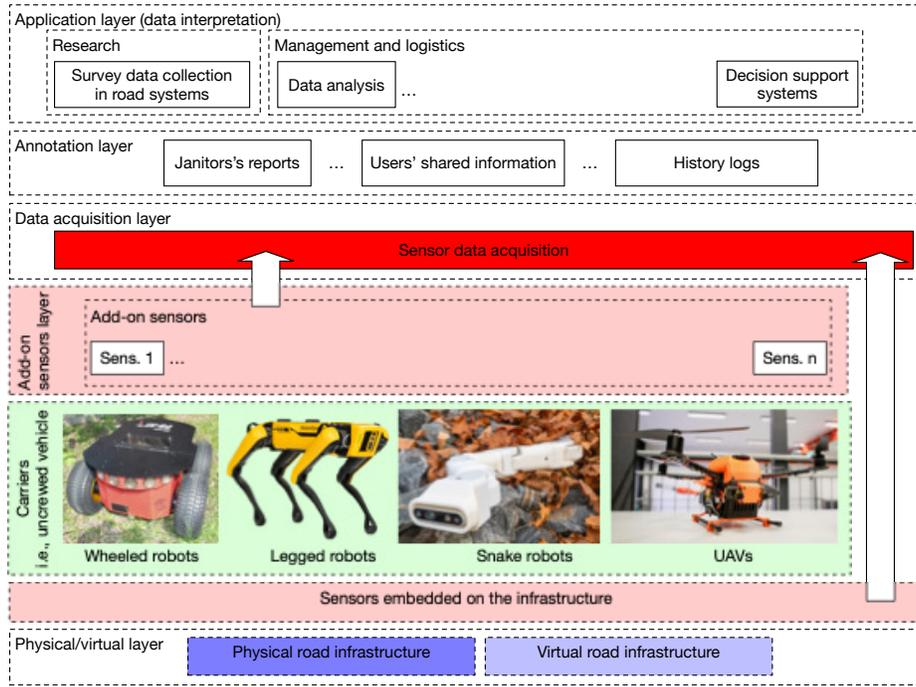
**Fig. 2.** The universal framework for creating a digital twin for the road infrastructure.
